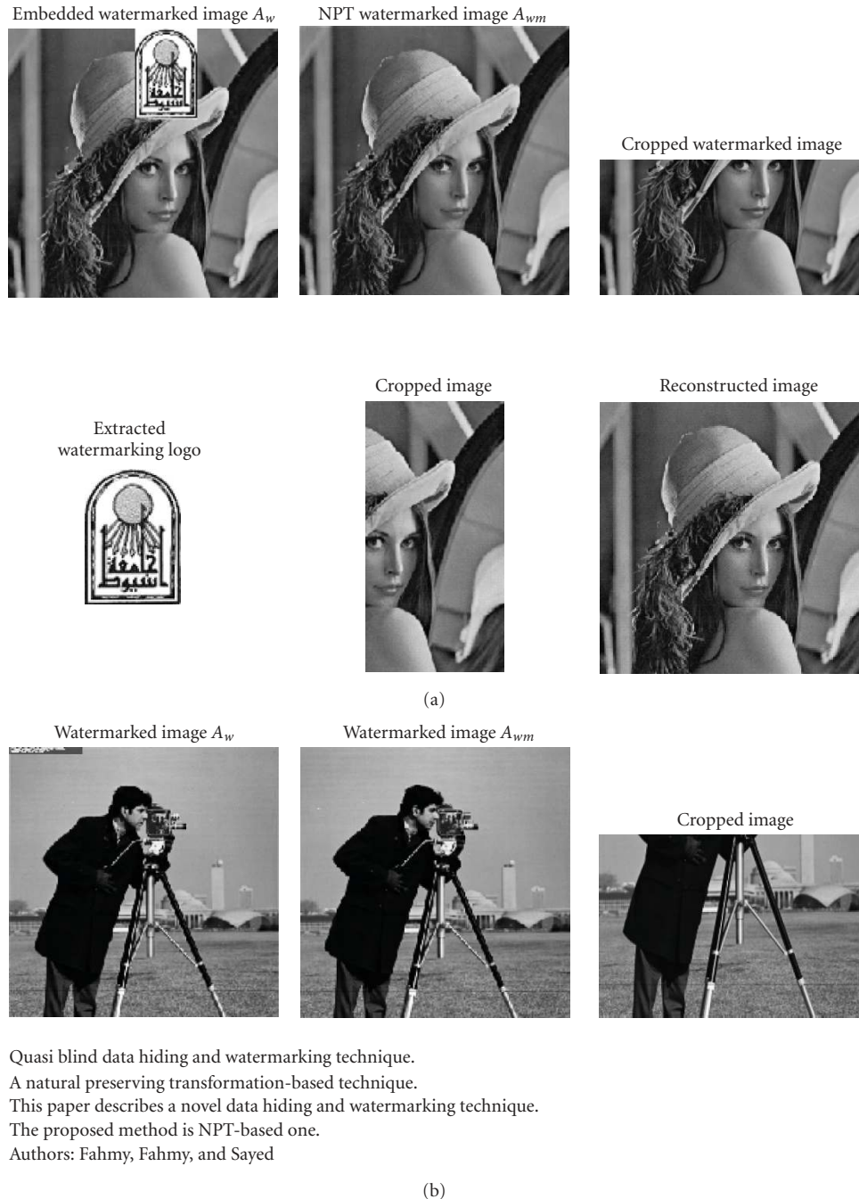
FIGURE 7: (a) Cropping performance of optimum location embedding, together with the extracted logo. \alpha = 0.99 , NCORR = 1 and SNR = 39.23 dB. (b) Cropping of top embedded Cameraman image, together with the text. \alpha = 0.99 .
