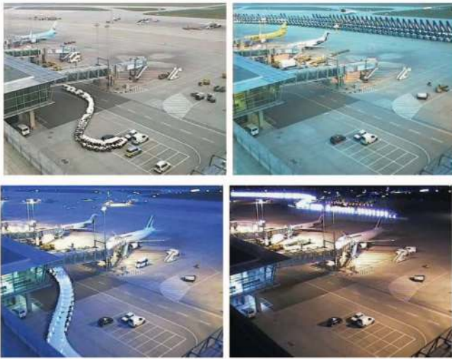
Fig. 7. Four extracted tubes shown “flattened” over the corresponding backgrounds from Fig. 6. The left tubes correspond to ground vehicles, while the right tubes correspond to airplanes on the runway at the back. This figure is best viewed in color.
