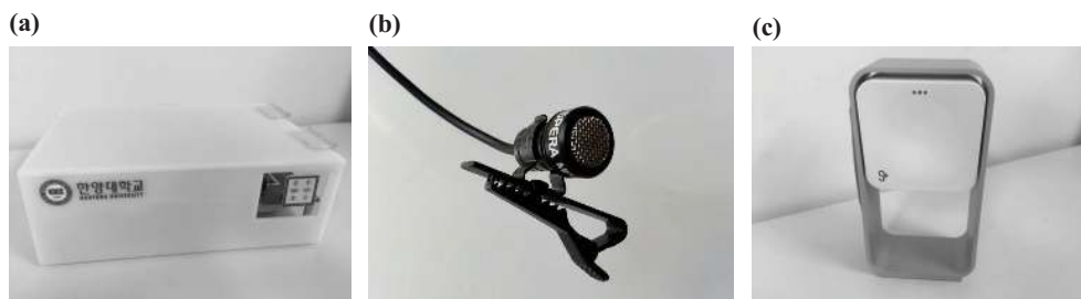
Figure 6. The devices used in experiment: (a) RFbeam K-LC5 Doppler radar sensor and ST-200 evaluation system; (b) OPERA MP-06 directional microphone sensor; (c) ResMed S+.
