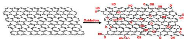
Figure 3. Oxidation of graphene sheet to form graphene oxide.
