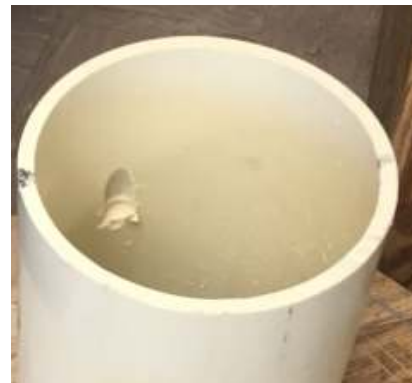
Fig. 7. PVC pipe with internal damage.
