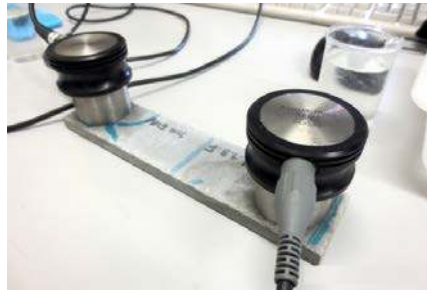
Figure 5. Test setup for UGW experiments
