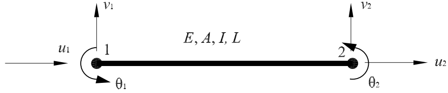
Figure 4.8: A frame element and its nodal d.o.f.
