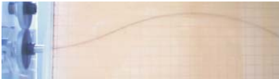
Fig. 7. (Top) The bicycle nonholonomic model prediction for a run with two curves, shown with average data (including nuisance parameters) and standard deviation bars. (Bottom) During the experiment, the needle was inserted 8.3 cm, spun 180°, then inserted another 16.7 cm.
