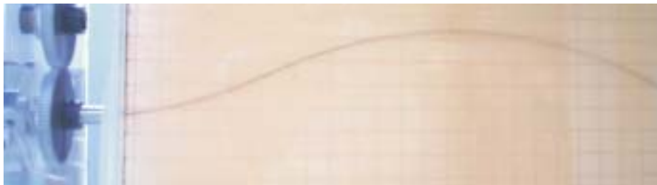
Fig. 9. (Top) The unicycle nonholonomic model prediction for a run with two curves, shown with average needle path data (including nuisance parameters) and standard deviation bars. The single parameter model is not able to fully capture the curvature variations of the physical needle. (Bottom) Photograph of one needle insertion.
