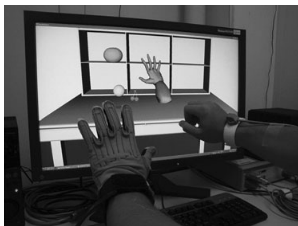
Figure 1 A personal-computer-based desktop virtual reality system for mirror visual feedback therapy. The arm on the affected side (right) and the targets appear in the virtual environment. Finger motion is simulated by the CyberGlove on the non-affected side (left) and arm motion is simulated by FASTRAK on the affected side.
