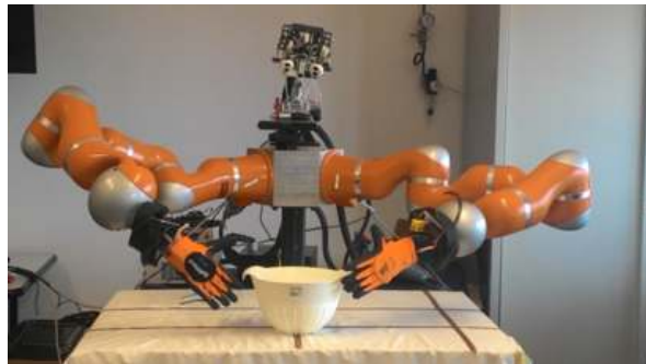
Fig. 1. VITO robot from research center “E Piaggio” at University of Pisa. This system is composed by two KUKA LWR arms controlled with compliance control. A PISA/IIT soft hand is mounted on each arm.
