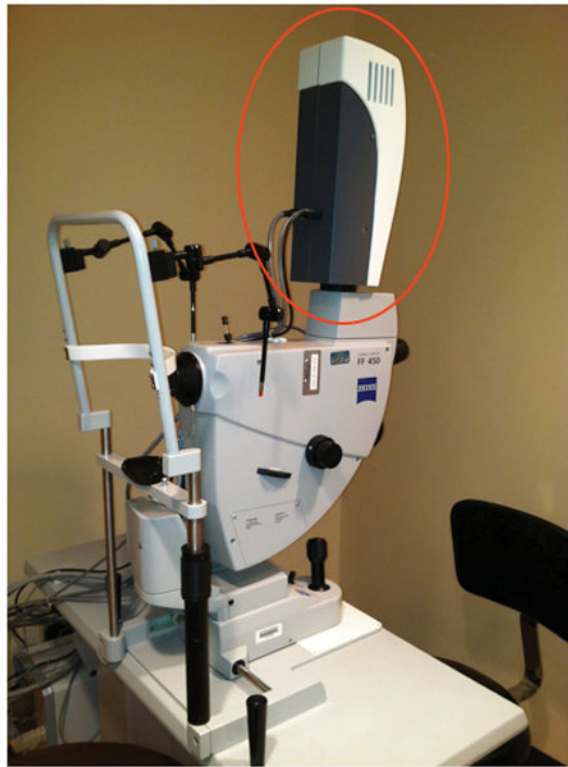
Figure 1. Hyperspectral computed tomographic imaging spectrometer (HCTIS) mounted on top of a standard Zeiss FF450 fundus camera. The HCTIS device is small and easily adaptable to the top port of the fundus camera. Images are acquired using the standard flash and trigger mechanism on the fundus camera. Images are saved on a laptop computer (not shown). Image processing and analysis are done with custom software as described previously [20–22].
