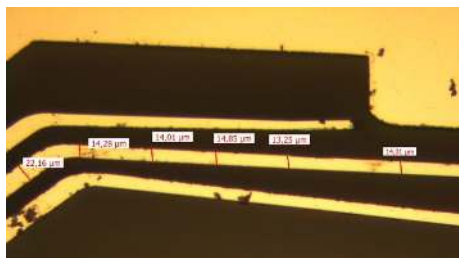
Figure B.7: Top view of the angled spring with improved dummy protective structures.
