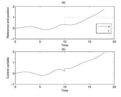
**Fig. 6** Oscillatory reference. (a) Tracking of reference r with  $q(x(t)) = (1 + x^2)/2$ ,  $r = 0.5 \sin(t)$ , (b) control variable u. Note that the controller with  $\lambda_{1,2} = -5$  does not track r(t) accurately. Compare this performance with the controller in Fig. 7(a)
