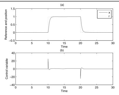
To obtain the value of the feedforward gain, we match closed-loop dc gain  $H_{CL}(0) = -C(A - BK)^{-1}BG$  with the open-loop dc gain  $H_{OL}(0) = -CA^{-1}B$  [40]. For the open-loop case,  $H_{OL}(0) = 1$ . For the closed-loop,  $H_{CL}(0) = \frac{1}{25}G$ . Thus, to match the dc gains, we choose G = 25 as the value of the gain associated with the reference.
