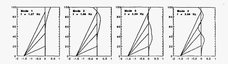
Fig. 2. Frequencies and mode shapes of first four natural modes of stack
