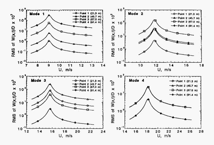
Fig. 3. RMS values of stack motions as a function of wind speed
