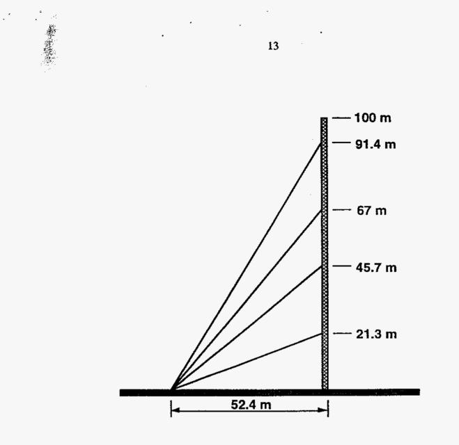
Fig. 1. Stack supported by guy wires at four levels
