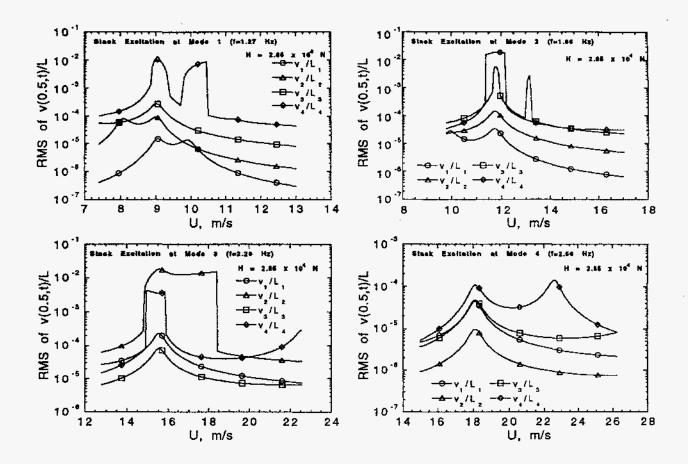
Fig. 5. Nondimensional RMS displacements of cable at  $x/\ell = 0.5$
