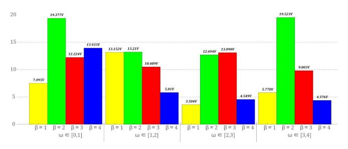
**Figure 17.** Comparison of the efficiency of harvesting energy in selected bands of variability of the dimensionless excitation frequency  $\omega$ .
