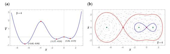
**Figure 14.** The localization of fixed points is shown as (**a**) potential characteristics, (**b**) phase plane with the corresponding homoclinic orbits and vector fields.
