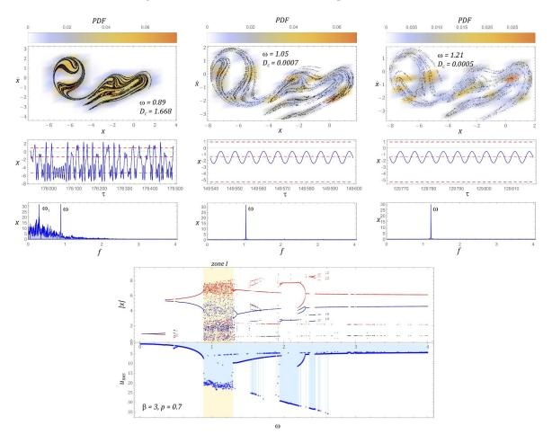
**Figure 12.** Bifurcation diagram correlated by the frequency spectra with the diagram of RMS voltage output induced on piezoelectric electrodes and examples of chaotic responses (Poincaré maps with correlation dimension and probability density function (PDF) indicated).
