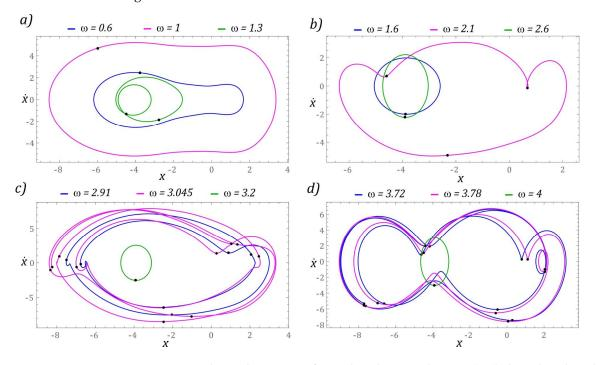
**Figure 10.** Sample graphic images of periodic solutions. The cases (**a**–**d**) show the selected solutions for increasing  $\omega$ . The corresponding Poincaré maps with multiple black points indicate higher period solutions.
