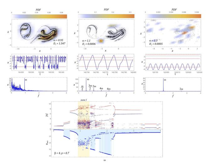
**Figure 15.** Bifurcation diagram correlated by the frequency spectra with the diagram of RMS voltage output induced on piezoelectric electrodes and examples of chaotic responses (Poincaré maps with correlation dimension and probability density function (PDF) indicated).
