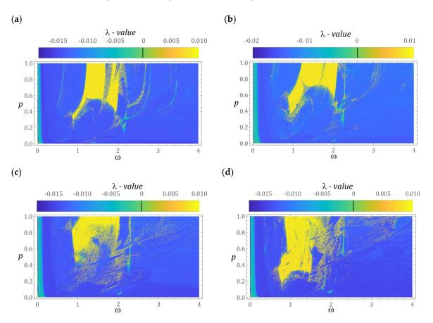
**Figure 4.** Influence of  $\beta$  on the distribution of the largest Lyapunov exponent,  $\lambda$ , for various geometrical factors,  $\beta$ : (a)  $\beta = 1$ , (b)  $\beta = 2$ , (c)  $\beta = 3$ , and (d)  $\beta = 4$ .
