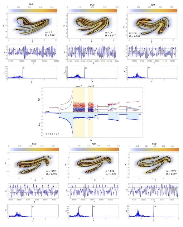
**Figure 6.** Bifurcation diagram correlated by the frequency spectra with the diagram of RMS voltage induced on piezoelectric electrodes and examples of chaotic responses (Poincaré maps with correlation dimension and probability density function (PDF) indicated).
