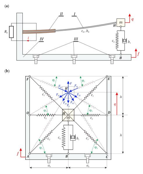
**Figure 1.** Schematic diagrams of the energy harvesting system with a star-shaped structure of elastic elements, visible from the direction: (**a**) perpendicular to the axis of the flexible beam, (**b**) parallel to the axis of the flexible beam. Geometrical and system parameters as well as the resulting force with their components are denoted in the picture.
