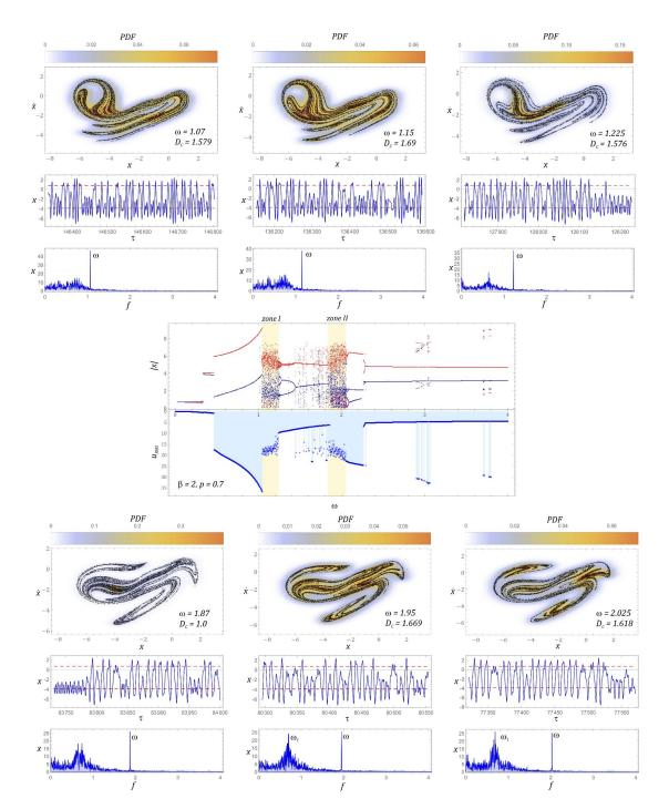
**Figure 9.** Bifurcation diagram correlated by the frequency footer with the diagram of RMS voltage induced on piezoelectric electrodes and examples of chaotic responses (Poincaré maps with correlation dimension and probability density function (PDF) indicated).
