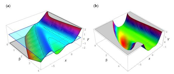
**Figure 2.** Three-dimensional images: (a) mechanical characteristics (restore force, *F*), (b) potential barrier, *V* versus tip mass displacement, *x*, and the geometrical parameter,  $\beta$ .
