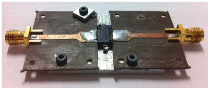
Fig. 4. LDMOS transistor mounted on the PCB board for the low-frequency characterization.
