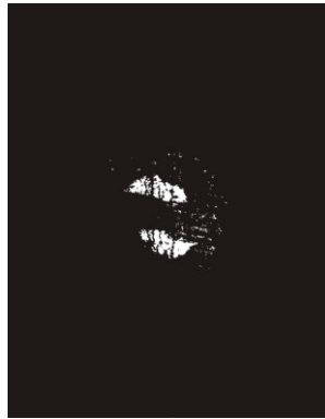
Figure 5 Image of the defect using ultrasonic C-Scan
