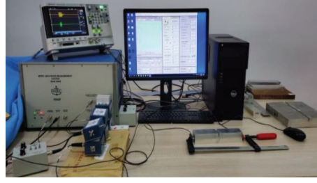
FIGURE 7: Experimental platform setup of nonlinear Lamb detection.
