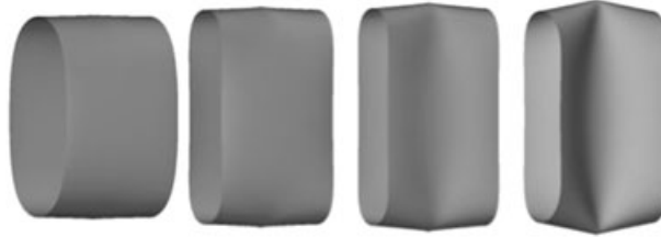
Figure 14. Selected snapshots of the deformation process during the pullout of an open-ended cylindrical shell (deformation not magnified), showing the buckling event for a force of about 2 \cdot 10^4 .
