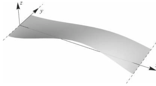
Fig. 2 Deformable plate, moving across a domain, bounded by two lines ( dashed ): three-dimensional view
