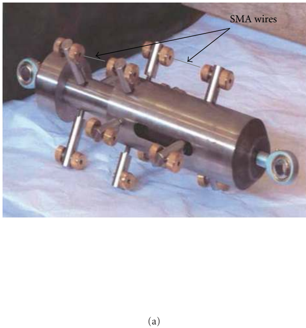
FIGURE 2: Shape memory alloy damper device. (a) Schematic. (b) Force displacement relation.
