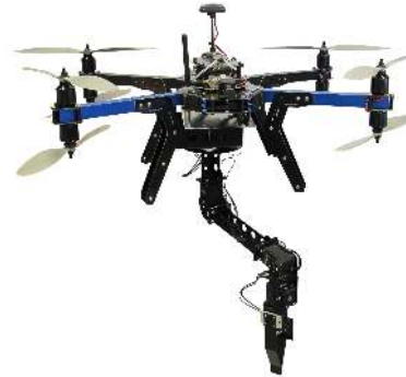
Fig. 1. Aerial manipulator, used in the experiments, consisting on a 3DR-X8 coaxial multirotor platform with a custom-built 3 degrees-of-freedom serial arm attached below.
