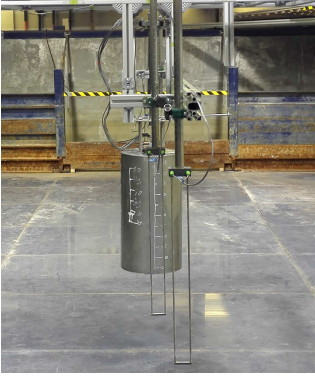
Fig. 1. A 1/50 PAWEC prototype installed for wave tank tests.
