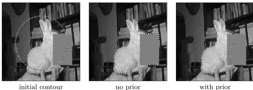
Fig. 9. Begin of the tracking sequence: initial contour, segmentation without prior, segmentation upon introducing the nonlinear prior on the contour.
