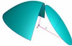
Figure 2: Geometrical Surface of off-axis Parabolic reflector
