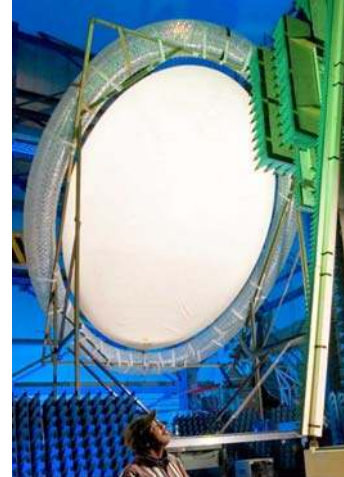
Figure 3. 4x6 meter full scale parabolic reflector antenna.
