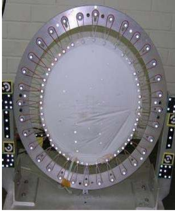
Figure 1. 0.3 meter reflector antenna dish mounted on a frame.
