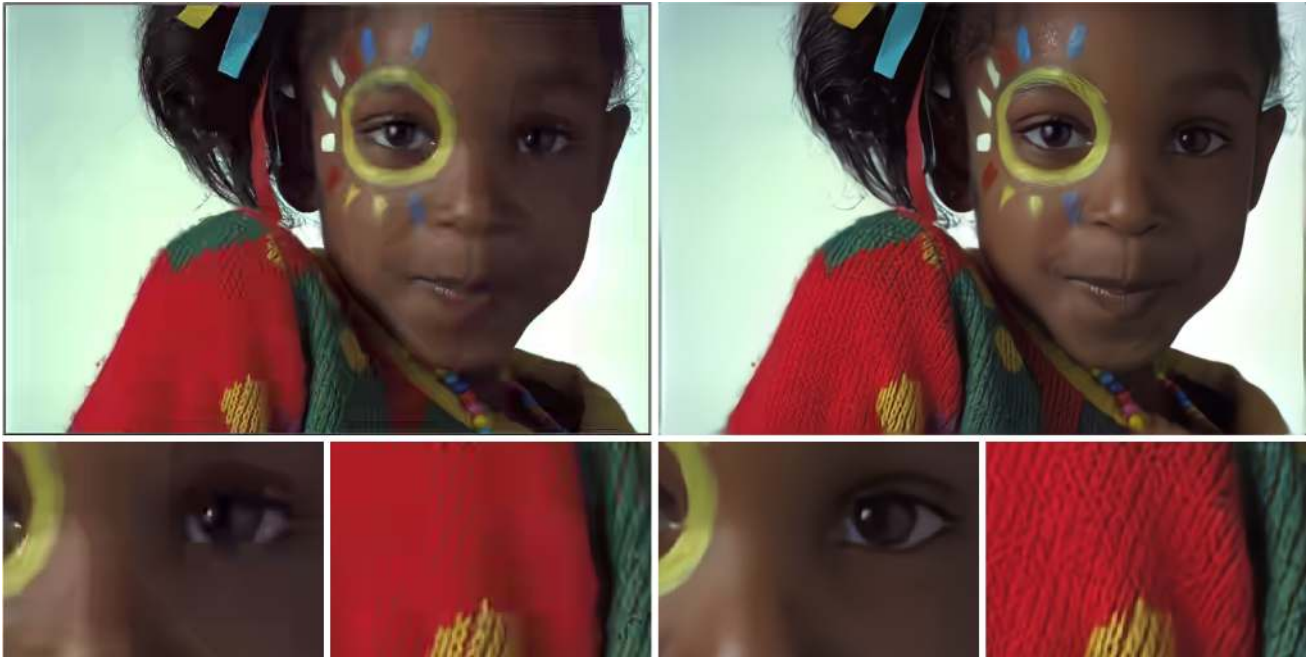
Fig. 14. Reconstructions of kodim15 [34] compressed by BPG (left, 0.0738 bpp) and by a learned NTC model [33] optimized for MS-SSIM (right, 0.0713 bpp). The combination of NTC and an MS-SSIM loss function, which is designed to model texture masking effects in the human visual system, leads to significantly better texture retention in the sweater and fewer geometric distortions on the person's face.
