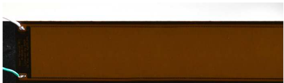
Fig. 4 Section of the MFC patch (orange colour) bonded onto the composite specimen (black). (Color figure online)
