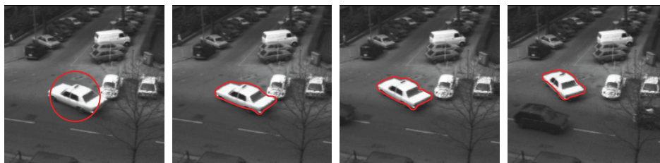
Figure 17. Segmentation of a moving car with our NL-N model (3.6) and the motion distance (8.1). Initial curve (first column) on the first frame and final curves (second–fourth columns) on the first, 13th, and 31st frames of the sequence are shown. Parameters: n = 191 , \tau = 11/n , (\sigma, \xi) = (\infty, 41/n) , \gamma = 0.005/n .
