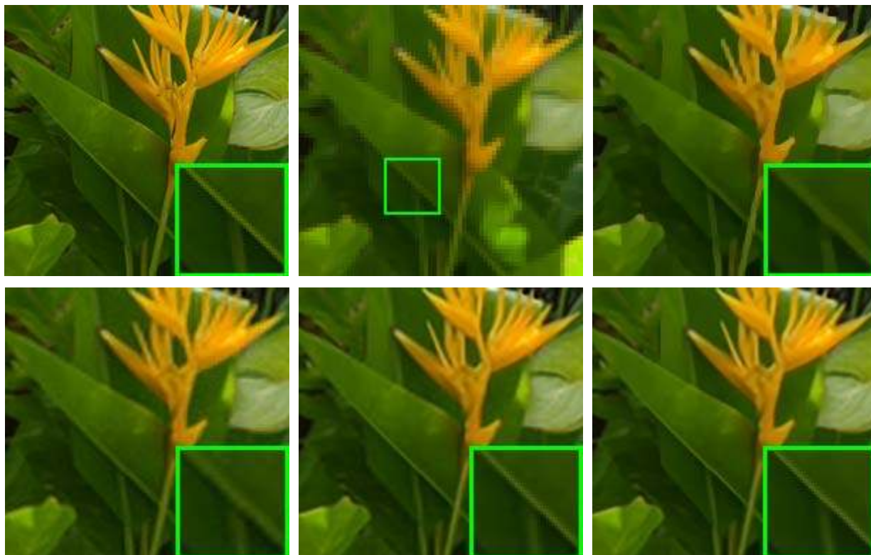
Figure 9: Image super-resolution performance comparison on Plant image (scaling factor 3, \sigma_n=0 ). From left to right and top to bottom: original image, LR image, the reconstructed images by TV [26] (PSNR=31.34dB; FSIM=0.8909), sparsity-based [23] (PSNR=31.55dB; FSIM=0.8964), ASDS-Reg [21] (PSNR=33.44dB; FSIM=0.9242), and the proposed NCSR (PSNR= 34.00dB; FSIM= 0.9369).
