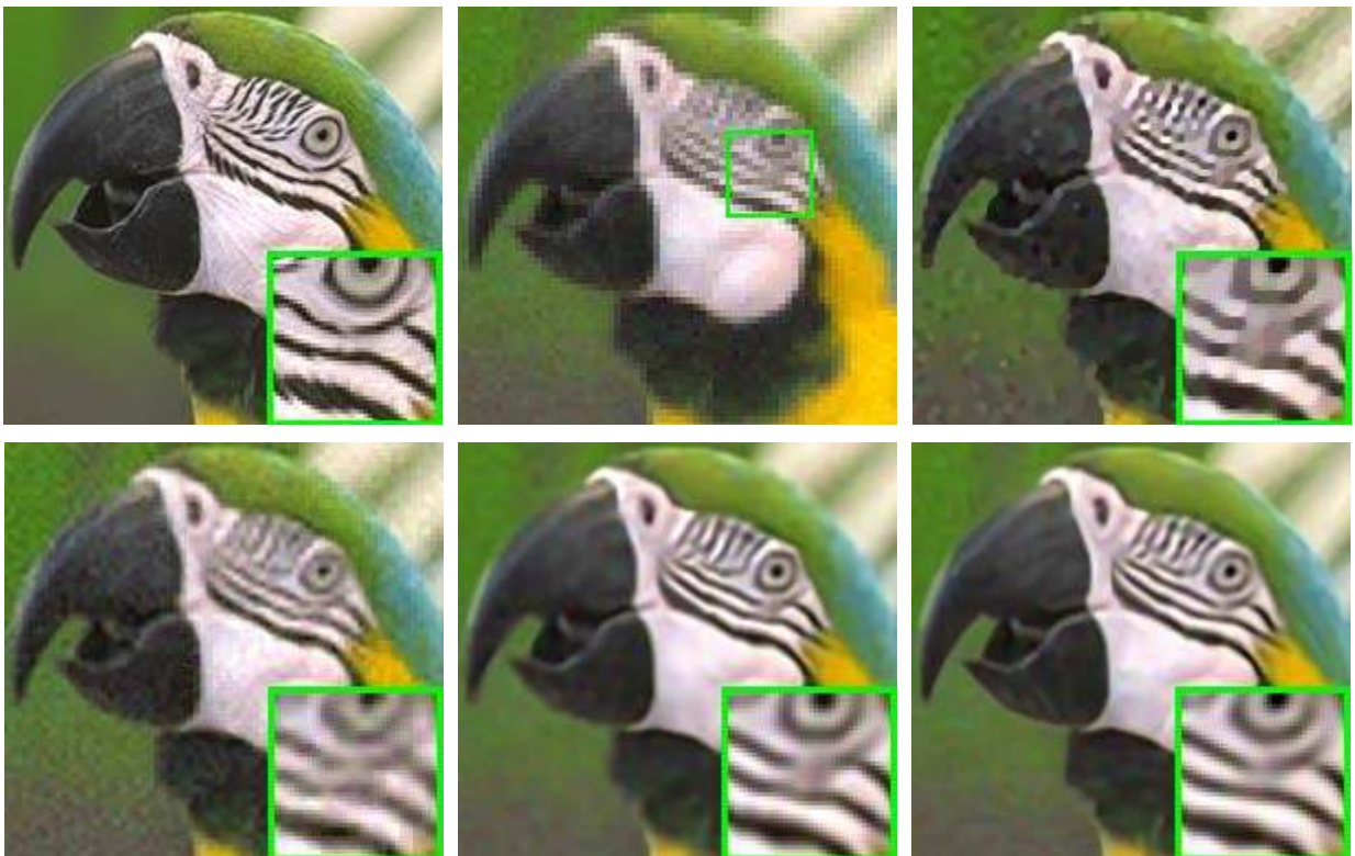
Figure 11: Image super-resolution performance comparison on Parrot image (scaling factor 3, \sigma_i=5 ). From left to right and top to bottom: original image, LR image, the reconstructed images by TV [26] (PSNR=27.01dB; FSIM=0.8562), sparsity-based [23] (PSNR=27.15dB; FSIM=0.8632), ASDS-Reg [21] (PSNR=29.01dB; FSIM=0.9182), and the proposed NCSR (PSNR= 29.51 dB; FSIM= 0.9210 ).
