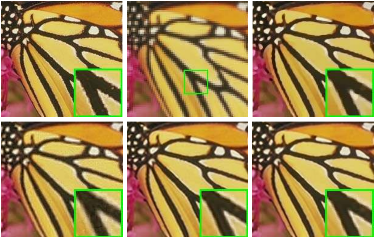
Figure 10: Image super-resolution performance comparison on Monarch image (scaling factor 3, \sigma_i=0 ). From left to right and top to bottom: original image, LR image, the reconstructed images by TV [26] (PSNR=26.57dB; FSIM=0.8970), sparsity-based [23] (PSNR=24.70dB; FSIM=0.7995), ASDS-Reg [21] (PSNR=27.28dB; FSIM=0.8789) and the proposed NCSR (PSNR= 28.10 dB; FSIM= 0.9031 ).
