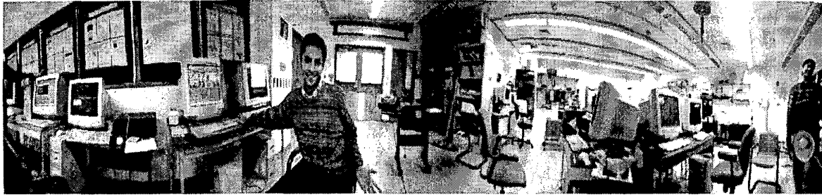
Figure 7: Panoramic video stream generated using the polycamera shown in Figure 6. The 360 degree panorama is computed using a look-up table, which is constructed taking into account the relative orientations of the four wide-angle cameras as well as their distortion parameters. Notice at extreme right, the extended hand gets warped to the left of the panoramic image.
