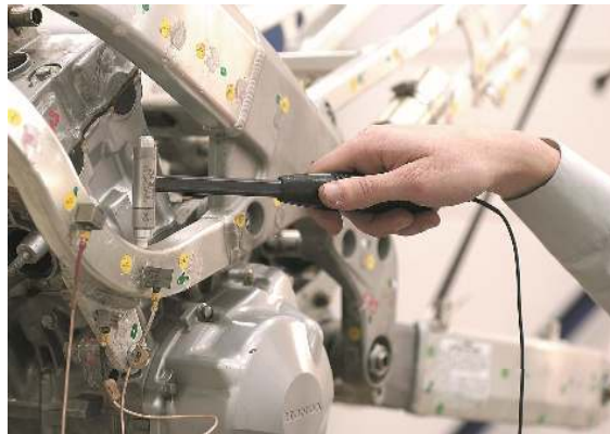
Figure 16. Hammer excitation in a mechanical vibration analysis in the vibration labs of Siemens Industry Software Leuven, Belgium. A force transducer is put in the tip of the hammer, allowing the impact force to be measured. Accelerometers are mounted on the mechanical structure to measure the response of the system.
