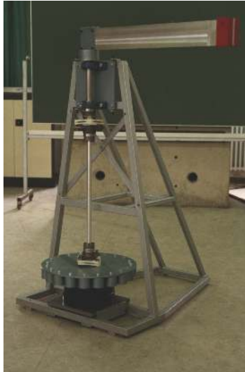
Figure 5. The one degree-of-freedom flexible robot arm of the KULeuven PMA department of Mechanical Engineering. The red mass at the tip of the flexible arm is driven by an electric motor. The input signal is the motor current, the output signal is the acceleration measured at the tip of the robot. A periodic excitation signal is used, the period length is N = 4096 with f_s = 500 Hz, and P = 10 periods are measured in steady-state conditions. Only the odd frequencies [1, 3, \dots, 201]f_0 , with f_0 = f_s/N = 0.1221 Hz are excited.
