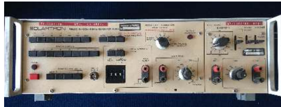
Figure S10. Pseudo random binary signal generator from the 1960's, used for example in laboratories at the School of Engineering, University of Warwick. Dedicated generators to generate MLBS and related signals, like the inverse repeat binary sequence, were built and commercialized. Besides the original signal u(t) , also a copy with a user adjustable delay u(t-\tau) was generated. This allowed the correlation y(t)u(t-\tau) to be measured using analog correlators, making a direct measurement of the impulse response g(\tau) possible.
