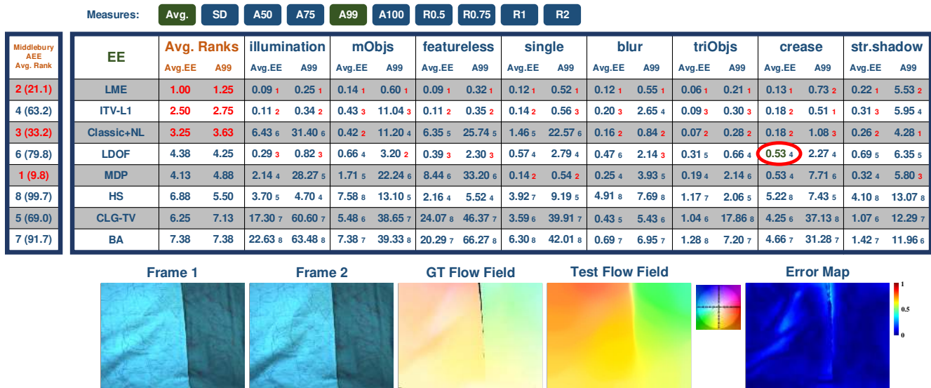
Fig. 6. Screen shot of our public evaluation website for RGB/Color based dense tracking/optical flow algorithms. Sample scores for the short sequences are shown, and we demonstrate the Endpoint Error (EE) evaluation. Multiple statistics/measures (Sec. II-C) can be manually selected on the top of the table and illustrated as sub-columns within a sequence where the subscripts show the rank in that sub-column. The user can mouse-click any of the results to show sequence details, the proposed flow field and the error map against the ground truth (as shown on the bottom row). All methods are listed in order of their average rank (Avg. Ranks).
