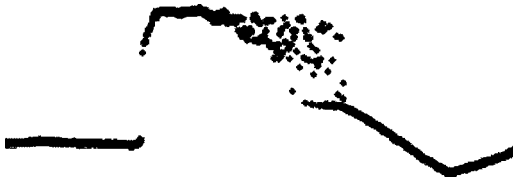
Fig. 1. Nonlinear resonance and oscillatory instability in optical microsphere observed in the experiment. Horizontal axis corresponds to detuning from the resonant frequency; vertical, output intensity.
