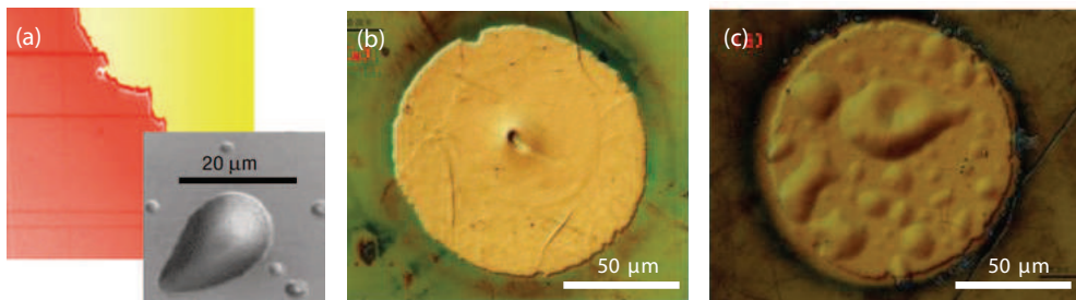
Fig. 11. Gas bubbles under the electrodes formed during the Forming processes of (a) the Pt/single crystalline SrTiO 3 /Pt memory cell (Szot et al., 2006), (b) Cu/GO/Pt memory cell with a GO thickness of 90 nm, and (c) Au/GO/Pt memory cell with a GO thickness of 30 nm
