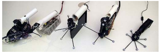
Figure 2: Five device prototypes (three NormalTouch versions and two TextureTouch versions) that we produced in our iterative process. Each design built on the learnings from the previous version, improving weight, robustness and mobility.
