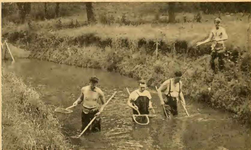
Minnesota Conservation Department crew making a fish census of a trout stream by the shocking method. The fishes are temporarily stunned by electricity passing from the electrodes held by each of the outside men.
