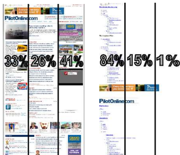
(a) When considering the entire page, the content of the page is distributed 33% in the left, 26% in the middle, and 41% in the right partitions when the stylesheet is present.
