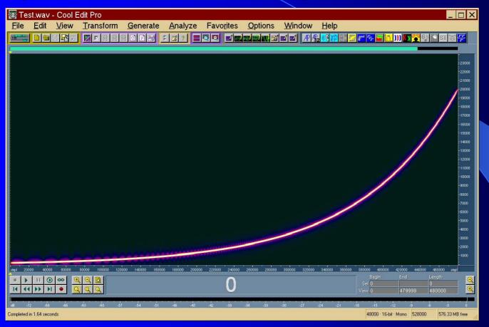
The excitation signal is a sine sweep with constant amplitude and exponentially-increasing frequency
