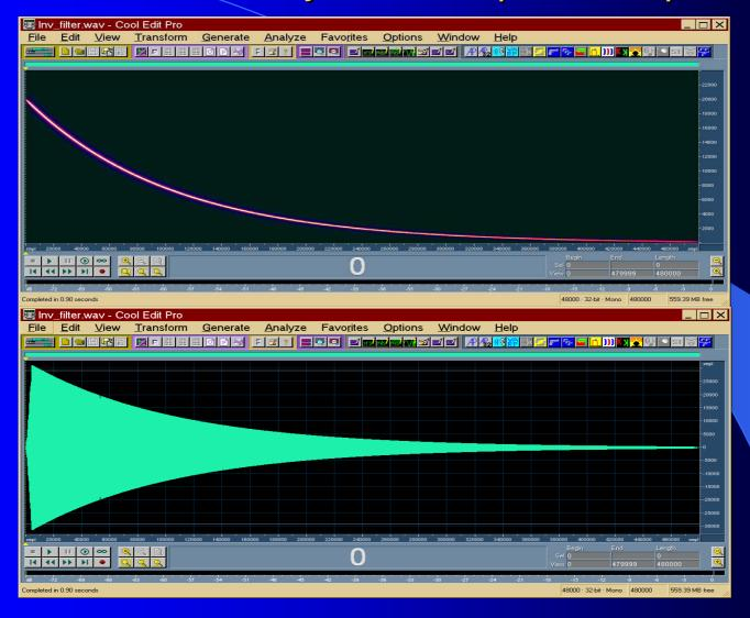
The deconvolution is obtained by convolving the raw response with a suitable inverse filter
