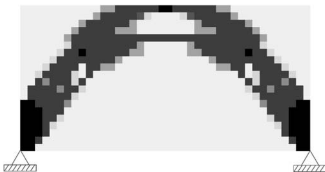
Fig. 14 Topology obtained by CONLIN at iteration 199 (modified SIMP law)
