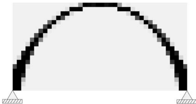
Fig. 13 Optimal topology for the arch problem when using GCMMA and the modified SIMP law
