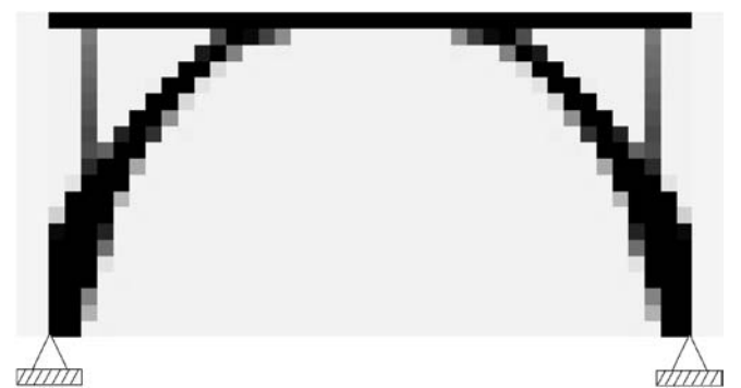
Fig. 19 Optimal topology for the bridge problem
