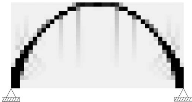
Fig. 11 Solution obtained with GCMMA for a minimum density of 0.01
