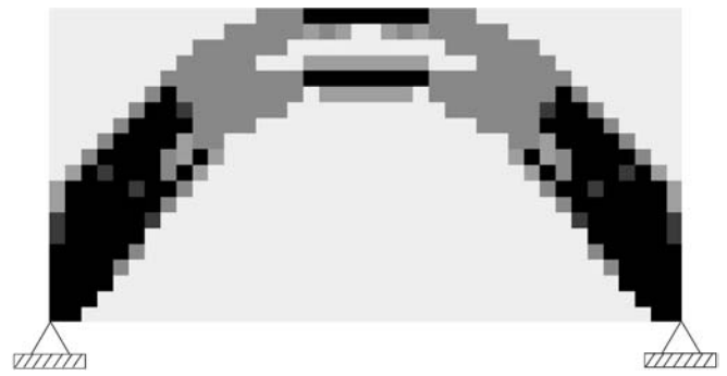
Fig. 15 Topology obtained by CONLIN at iteration 200 (modified SIMP law)
