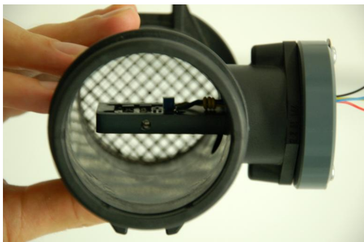
Figure 8. View of the interior of the automobile engine inlet tube with the air flow meter mounted in it.
