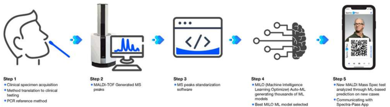
Figure 1. Conceptual drawing of study workflow. The study workflow consisted of patients providing a nasal swab specimen preserved in saline transport media. Media was tested by RT-PCR (Step 1) and swabs plated onto the MALDI-TOF-MS platform (Step 2). Mass spectra were standardized (Step 3) and then analyzed using machine learning via the Auto-ML MILO platform (Step 4). COVID-19 status is then exported to a smart device app (Step 5).
