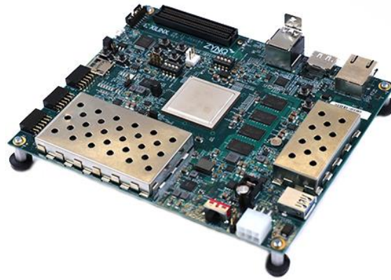
Figure 13. Photograph of the ZCU-104 evaluation board used to implement the routing algorithm.
