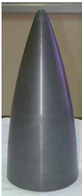
Figure 1. A digital photograph of sintered and machined thin walls (about 4 mm thick) of \beta -SiAlON prototype radome manufactured at ARCI, Hyderabad.
