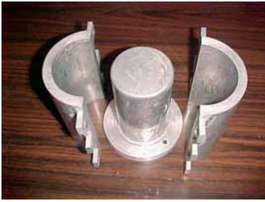
Figure 12. Split-type aluminium mould used for fabricating crucibles by following aqueous colloidal processing routes [19,59].
