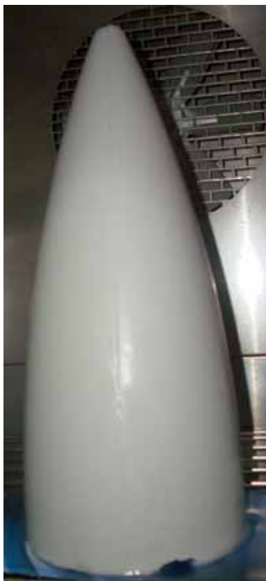
Figure 5. A green radome (about 290 mm height and 125 mm base diameter) consolidated from a 50 vol% of alumina-loaded slurry in a split-type Teflon-lined aluminium mould. This radome shape is made to demonstrate the net-shape consolidation capability of GCHAS colloidal processing route [10].
