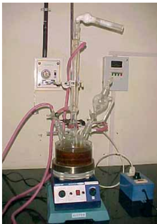
Figure 8. Experimental setup used for employing water-resistant coating on AlN as well as on \text{MgAl}_2\text{O}_4 spinel powders [15,43,47].
