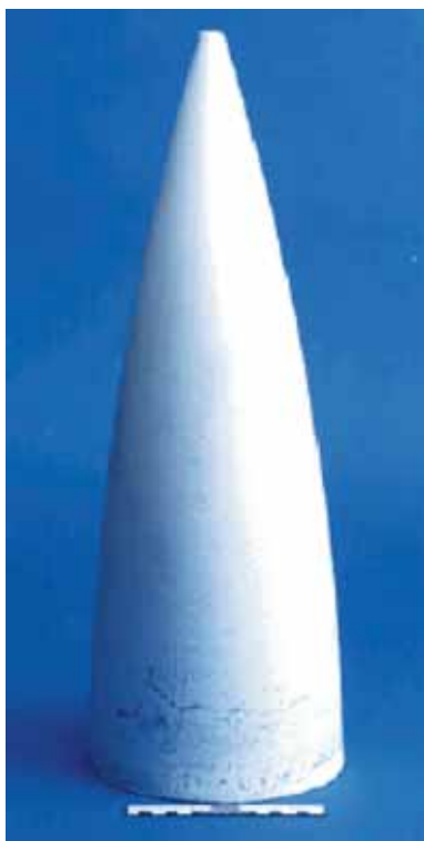
Figure 4. Photo of gelcast green body of radome manufactured by Janney et al [1], at Oak Ridge National Laboratory, USA. The presence of processing defects formed during setting of the slurry at the bottom portion of the radome can be noticed.
