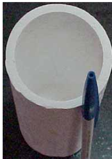
Figure 6. Dried green (not sintered) \text{MgAl}_2\text{O}_4 spinel crucible (500 ml capacity) consolidated by following an aqueous gelcasting of a slurry containing 45 vol% solids loading. This crucible shape is made to demonstrate the net-shape consolidation capability of GCHAS colloidal processing route out of water sensitive \text{MgAl}_2\text{O}_4 spinel powder. Prior to prepare colloidal suspension, the \text{MgAl}_2\text{O}_4 spinel powder was surface-passivated against hydrolysis by following a process developed at ARCI, Hyderabad [11–15].
