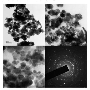
Figure 5. HR-TEM—SAED analysis of Cu-Zn-Mn mixed trimetal oxide nanoparticles.
