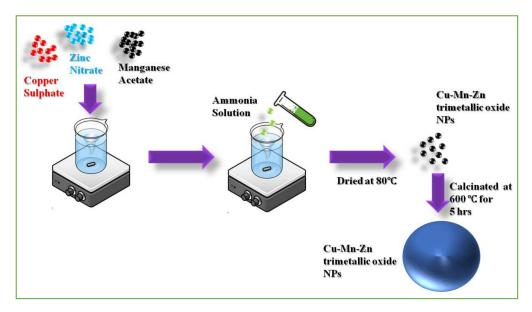
**Figure 1.** Synthesis of Cu-Zn-Mn mixed trimetal oxide nanoparticles (NPs).
