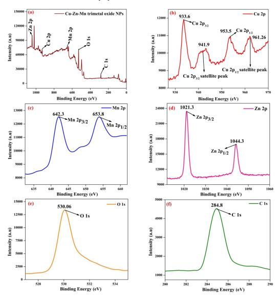
**Figure 6.** XPS of Cu-Zn-Mn mixed trimetal oxide nanoparticles. (a) survey scan of trimetal oxide; (b) Cu, (c) Mn, (d) Zn, (e) O, (f) C elements.
