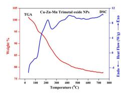
**Figure 10.** TG-DSC of Cu-Zn-Mn mixed trimetal oxide nanoparticles.
