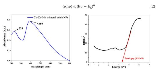
Figure 8. UV-Vis and Tauc plot of Cu-Zn-Mn mixed trimetal oxide nanoparticles.
