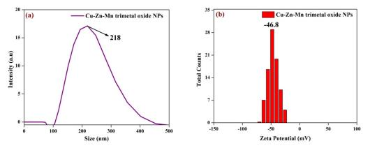
Figure 7. (a) Particle size and (b) Zeta potential of Cu-Zn-Mn mixed trimetal oxide nanoparticles.
