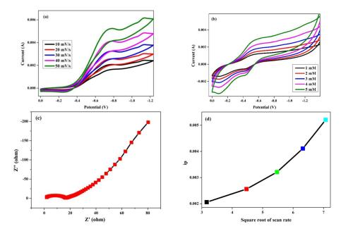
**Figure 11.** (a) CV graph of Cu-Zn-Mn mixed trimetal oxide nanoparticles with different scan rates, (b) CV graph with glucose at different concentrations, (c) Nyquist plots of the Cu-Zn-Mn mixed trimetal oxide, (d) plot of peak current vs. square root of scan rate.
