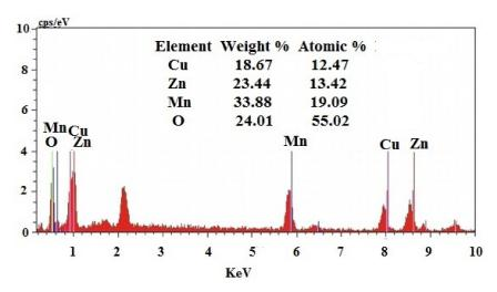
Figure 4. EDAX of Cu-Zn-Mn mixed trimetal oxide nanoparticles.
