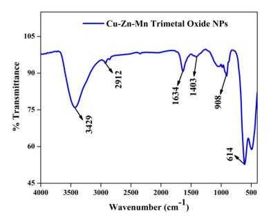
Figure 9. FT-IR of Cu-Zn-Mn mixed trimetal oxide nanoparticles.
