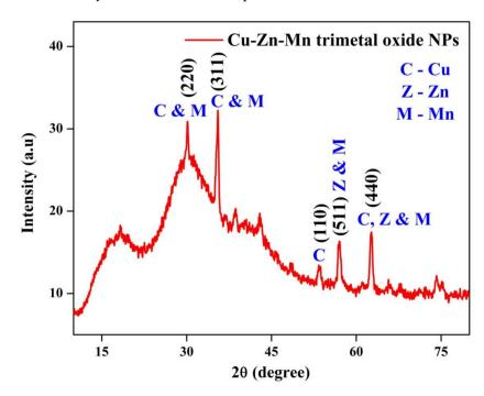
Figure 2. XRD pattern of Cu-Zn-Mn mixed trimetal oxide nanoparticles.
