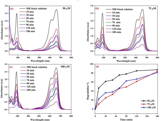
**Figure 12.** Photocatalytic degradation of methylene blue at (a) 50  $\mu$ M, (b) 75  $\mu$ M, and (c) 100  $\mu$ M. (d) Degradation efficiency of Cu-Zn-Mn trimetal oxide NPs.
