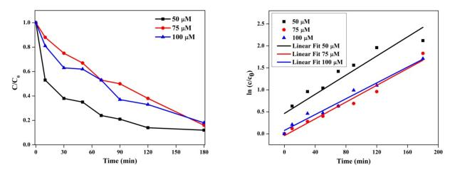
**Figure 13.** Plot of time vs.  $c/c_0$  and time vs.  $\ln c/c_0$  for photocatalytic degradation of methylene blue dye.
