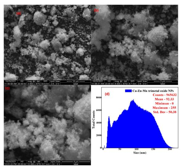
Figure 3. SEM of Cu-Zn-Mn mixed trimetal oxide nanoparticles. (a) 10  $\mu$ m; (b) 5  $\mu$ m; (c) 4  $\mu$ m; (d) size distribution.
