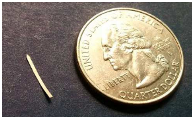
Fig. 13. Aluminum cantilever is fabricated separately from 100\text{-}\mu\text{m} aluminum sheet.
