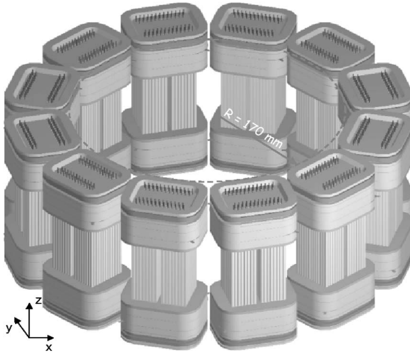
Fig. 3. A PET scanner comprising 12 camera modules with a free inner diameter of 34 cm, suited for brain diagnostics. The shape of the HPDs has been optimized to increase the active area coverage.
