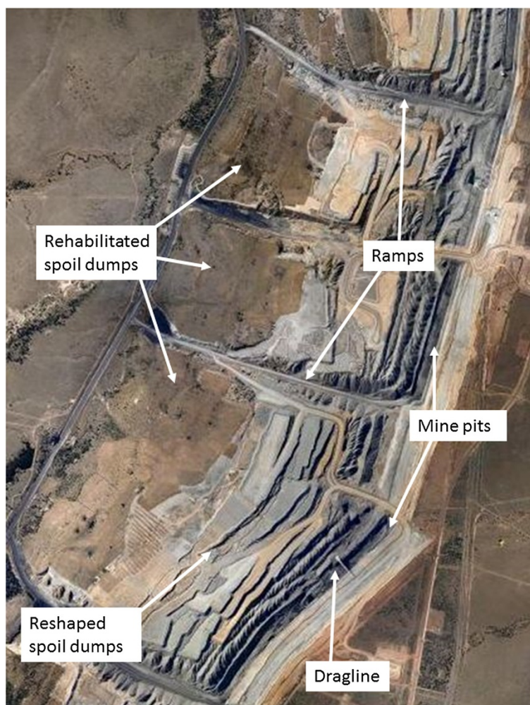
Figure 2 An overview of Blackwater coal mine operations and the location of rehabilitated spoil dumps in relation to the mine pits (image from AAM).
