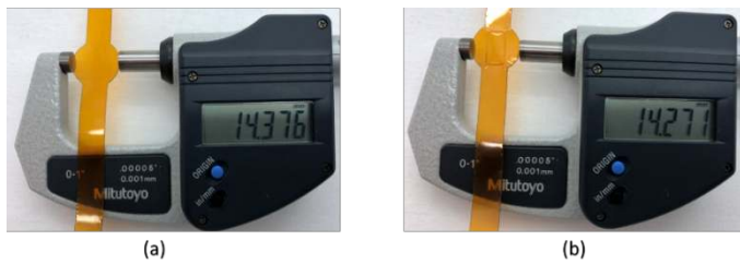
Figure 10. The diameter of circular feature for a Kapton film (a) before moulding and (b) after moulding.
