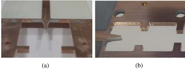
Fig. 8. Border metallization synthesizing the lateral walls of an ESIW. (a) 11 GHz prototype, (b) 19.5 GHz prototype.
