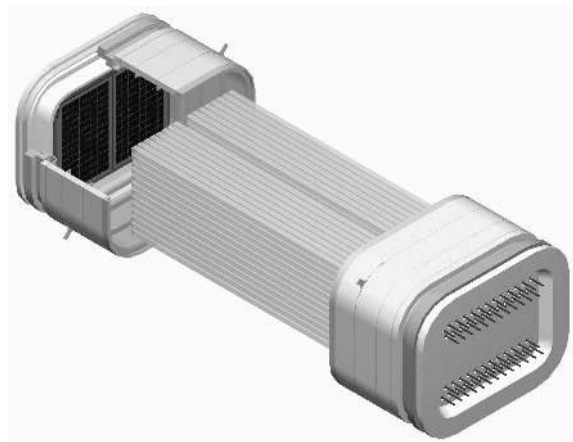
Figure 2. Drawing of a 3D axial detector module consisting of a matrix of 150 mm long crystals, read out by two HPDs.
