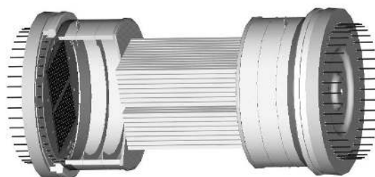
Figure 3. Prototype of a 3D Axial detector module for proof of principle measurements. The scintillator matrix is composed of already available YAP crystals of dimensions 3.2 \times 3.2 \times 100 mm 3 .
