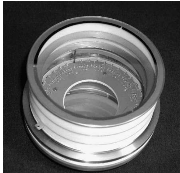
Figure 5. Photograph of a proximity focused prototype HPD with round silicon sensor and integrated front-end electronics.
